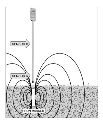
Figure 1: Detecting Magnetic Field of an Iron Marker
