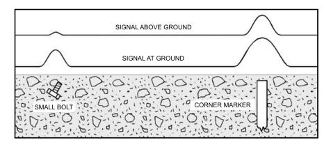
Figure 6: Raising the Locator Eliminates Unwanted Signals
