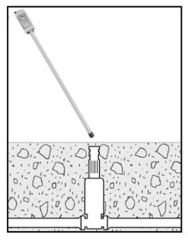
Figure 15: Locating Valve Boxes and Casings
