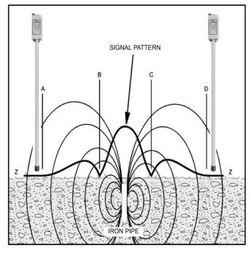
Figure 7: Signal Pattern from a Strongly Magnetized Marker
