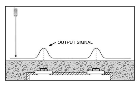
Figure 10: Signal Pattern Provided by Septic Tank Covers
