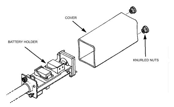
Figure 18: Exploded View of the Electronics Unit Cover
