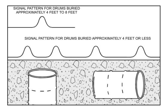
Figure 17: Signal Patterns Provided by Steel Drums
