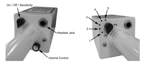
Figure 2: Sensitivity Set for Normal Range (position 2)
