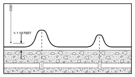
Figure 16: Signal Patterns Provided by Cast-Iron Pipes
