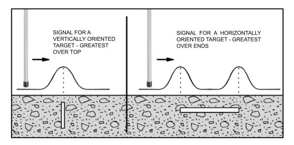
Figure 4: Signals from Vertical and Horizontal Targets
